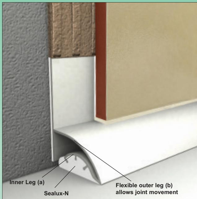
TRIMLUX combines a flexible pvc strip with Sealux-N silicone. The Sealux-N laid in the strip fuses with the Sealux-N laid on the ledge to form a watertight seal over the joint between the wall and the ledge.
