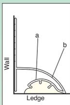
The Sealux-N silicone 'anchors' the inner leg (a) firmly to the ledge.
