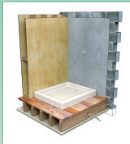
Semi-rigid acrylic baths and shower trays deflect when loaded with water and occupant causing the joint between the ledge and wall to expand
