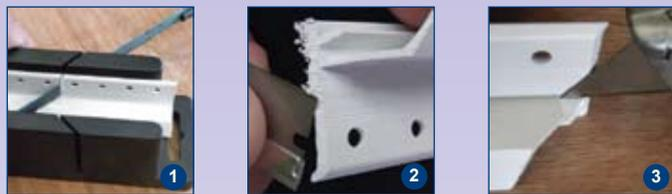
**1-7** 1. Measure and cut strips to length. Mitre cut corners. Square cut ends (refer to last paragraph). 2. Remove saw cut frays with a blade. 3-5. Notch each mitre cut with a snips or blade to form a square hole through meeting strips.
