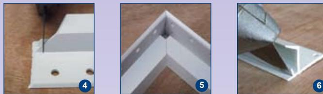
Test strips in position to ensure they fit correctly. 6-7. If outer strip edge is not resting on the ledge, score the strip with a blade and tear off removable inside leg.
