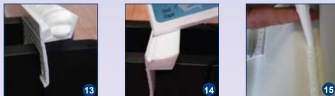
13-14. Insert first strip (middle strip if any) upside down into 2 mitre boxes (or similar support). Resting nozzle in strip, lay a 400mm line of Sealux-N inside the profile. Level Sealux-N across the strip with spatula. Redistribute or add sealant as required. Repeat process in 400mm steps until complete. Butter strip ends flush slightly proud with Sealux-N.
