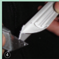
4 Pare off freys at cut ends
