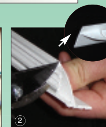
2 Mitre cut - snip inner leg as shown
